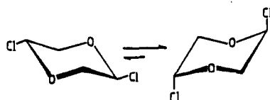
Figure 1. The anomeric effect: Electronegative substituents, attached to the anomeric carbon, prefer the axial setting, although from steric consideration alone the equatorial conformation would be favored.
